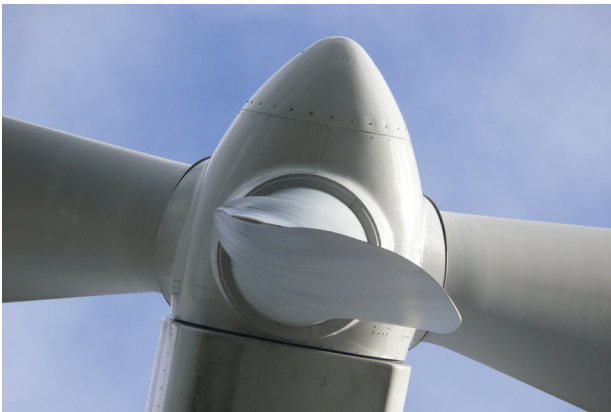
Rotor of a 2 MW wind turbine
